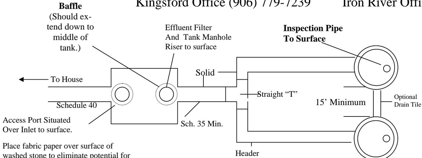
Place fabric paper over surface of washed stone to eliminate potential for fines to seep into stone.
